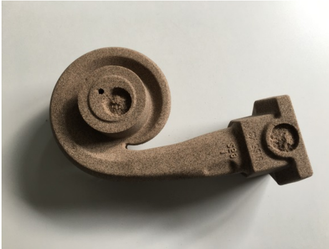
Image 7 – Sand core for a turbine housing
